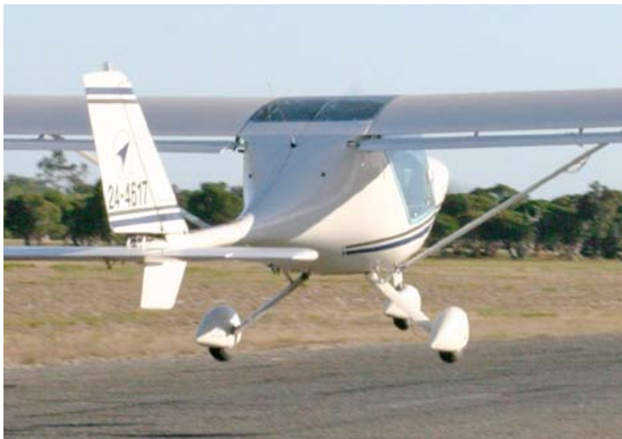
A broad aluminium tube acts as the rear fuselage and carries the tail, with a fibreglass fin and rudder of generous area and an all-flying tailplane or stabilator.
