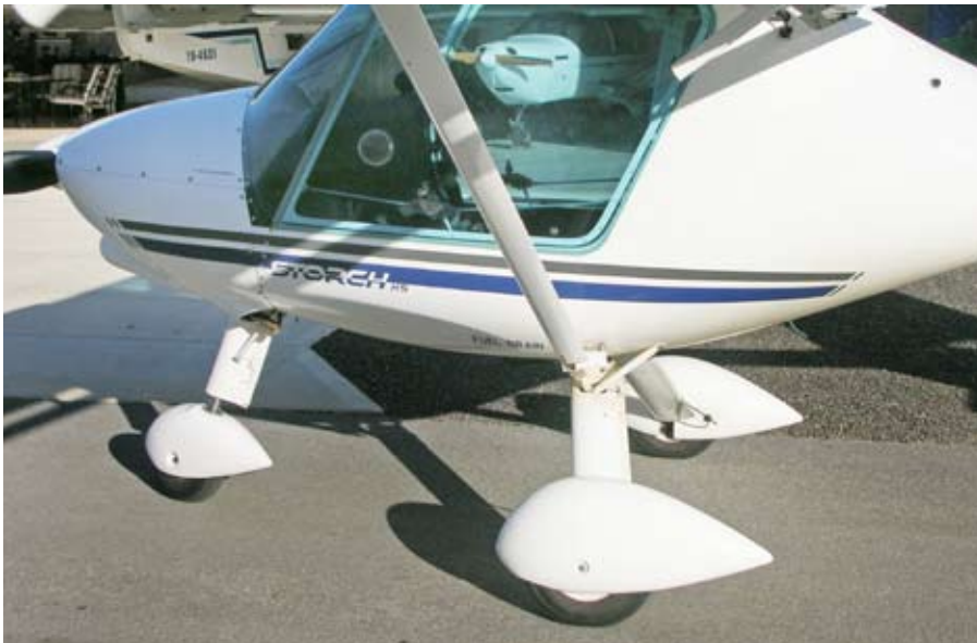
The Storch's simple and thick main landing gear legs can be unbolted and replaced in an hour or so – a very sensible feature for a training aeroplane.
