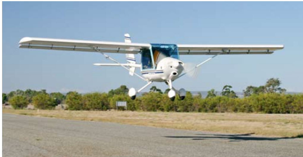
The author found it easiest to make all his approaches with full flaps and the throttle completely closed.
