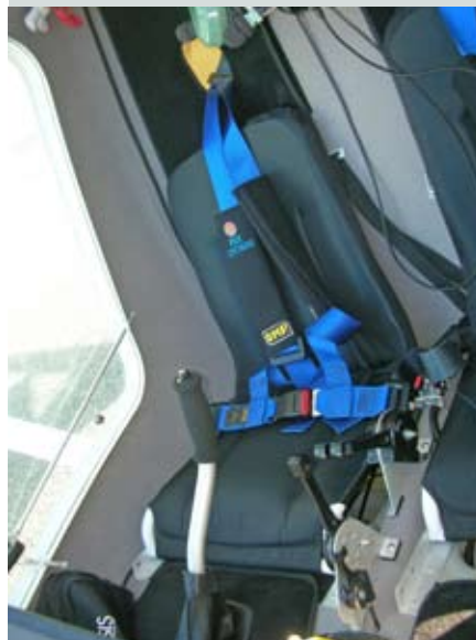
The seats offer good lumbar support despite rather thin padding, with fixed four-point harnesses.
